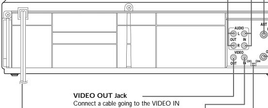
Connect a cable going to the VIDEO IN Jack of a camcorder, another VCR, or an audio-visual source (laser disc player, video disc player, etc.) here. *Details are on pages 32 and 38.*
